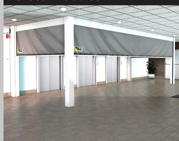
It may be required to create a protected lobby Smoke curtains can be used around the in front of a bank of elevator doors. Where this would previously have required the construction of a physical smoke and fire rated partition, a three sided lobby can now be produced using curtains.
